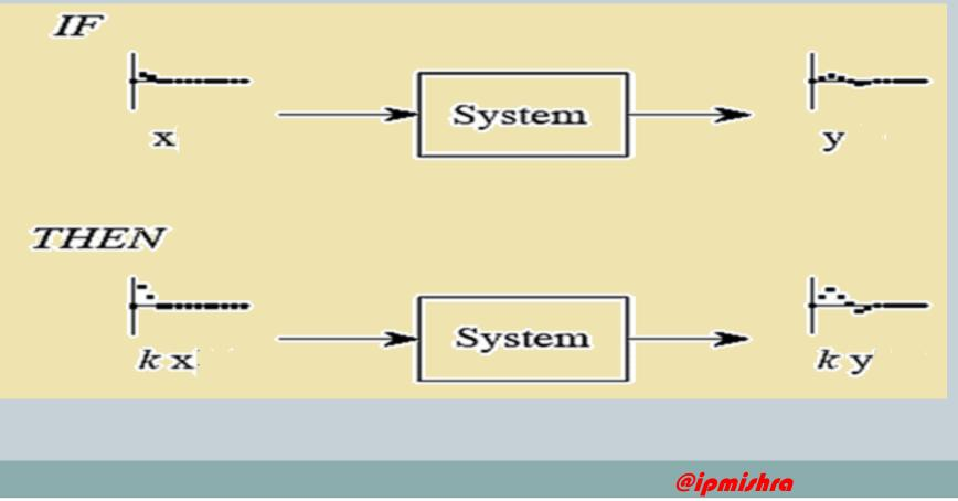
If, in a multi-input network the input x1 by itself yields output y1 and a second input x2 by itself yields y2, then the combination of inputs x1 and x2 yields the output y = y1 + y2.
