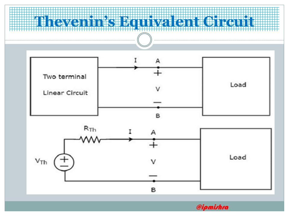
• Find the current flowing through 20  $\Omega$  resistor by first finding a Thevenin's equivalent circuit to the left of terminals A and B.
