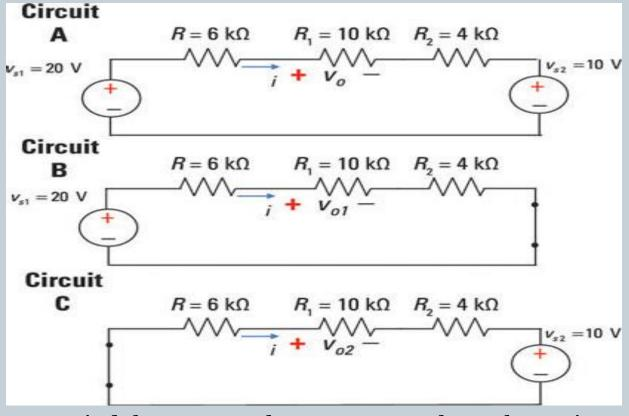
Find the output voltage Vo across the 10-k $\Omega$  resistor
